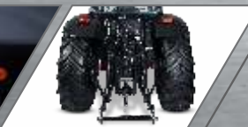
HYDRAULIC LIFTING CAPACITY 4500 KG
